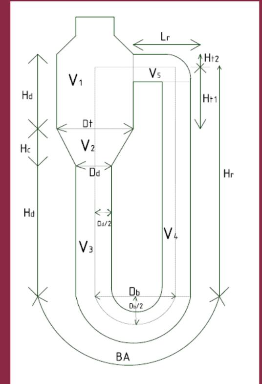
$$\underbrace{\frac{\pi(D_t/2)^2 H_t}{V_1}}_{V_1} + \underbrace{\frac{\pi H_c [(D_t/2)^2 + (D_d/2)^2 + D_t * D_d]}{3}}_{V_2} + \underbrace{\frac{\pi (D_d/2)^2 [H_d + BA + H_r + L_r]}{V_3 + V_4 + V_5}}_{V_3 + V_4 + V_5} = \underbrace{1,000,000}_{V_T} \quad (1)$$
